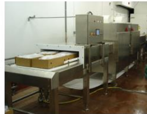
TMW75 Microwave Tunnel – used to defrost food -20°C to -2°C
